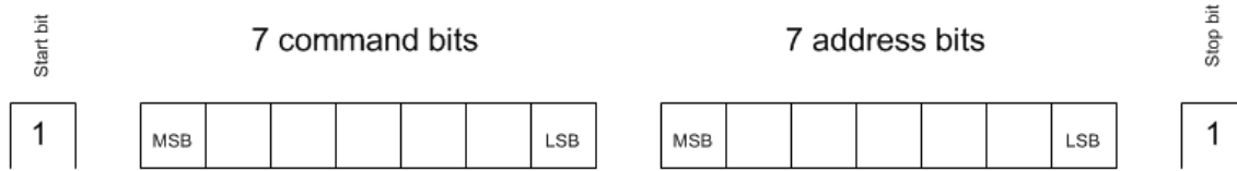
figure 1: 'Command signal' structure for power line communication (2 bytes)
