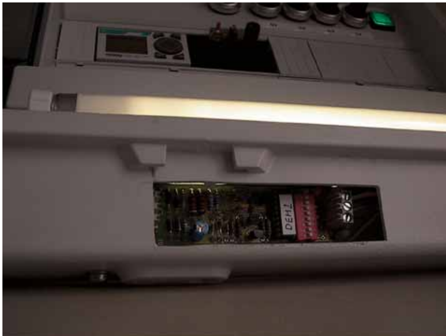
Vitolink receiver with 1-10 V dimming interface
